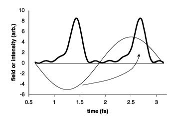
FIG. 3. Intensity envelope of the attosecond beats (thick line) and the IR pump field (thin line). The beat spikes, 266 as FWHM, occur 190 as after the field maxima. A wave packet ejected just after a peak of the field is recolliding with the nucleus (producing the XUV bursts) after about 1520 as.
