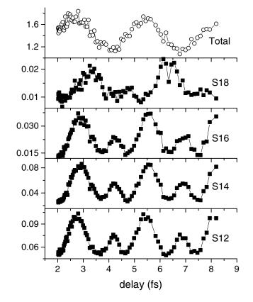
FIG. 2. Energy-integrated ionization signal (top panel) and sideband signals (from  $E_0 + 18\hbar\omega$  to  $E_0 + 12\hbar\omega$ ) vs the pumpprobe delay. Sideband signals were normalized to the corresponding total signal.
