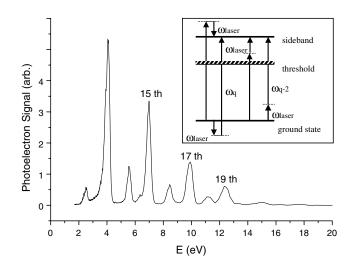
FIG. 1. Photoelectron spectrum of argon exposed to harmonics 11–19 and the IR probe. The single-photon peaks are labeled by the order of the harmonic. The sidebands appear in between. The inset shows the relevant quantum paths.
